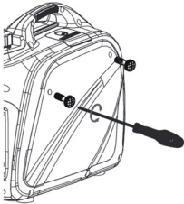
Figure 2-6. Remove Side Cover
