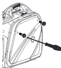
Figure 4-3. Remove Side Cover
